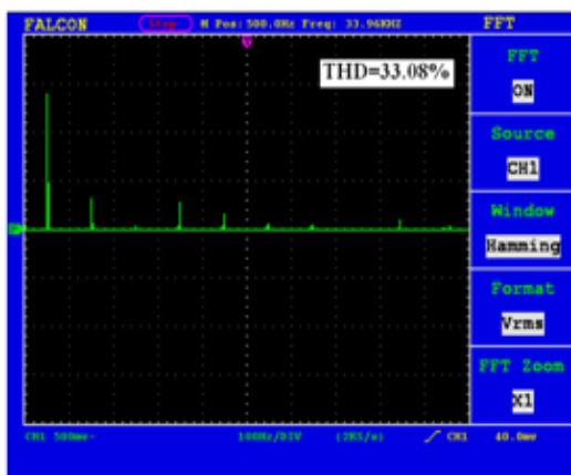
Fig10(a):-Harmonic analysis for 270W load
